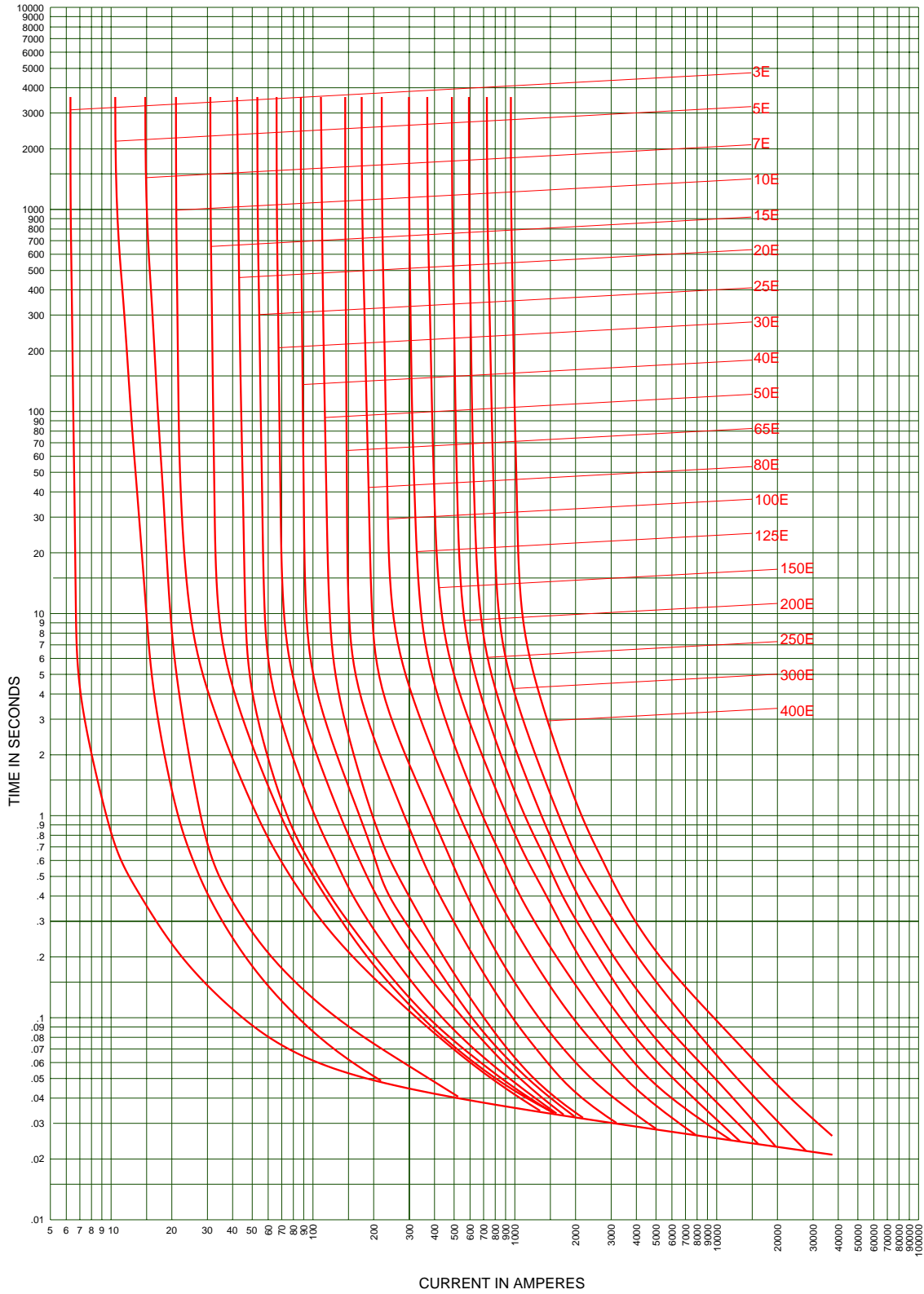
Type RBA-RDB-400 Refill Power Fuses - Standard Speed Refills Total Clearing Time-Current Characteristics - 2.4 to 34.5 kV
